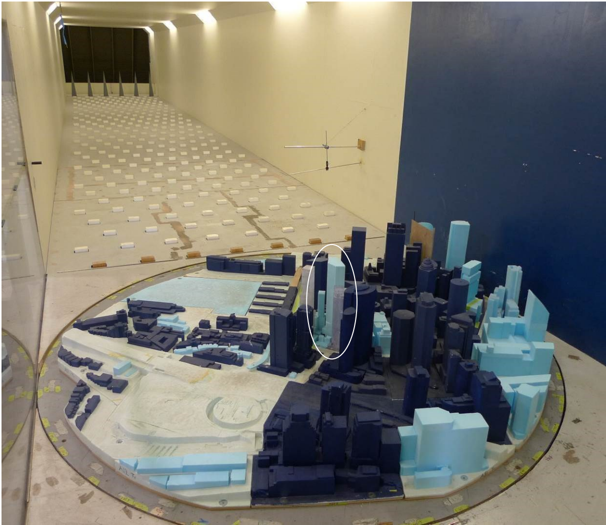
Figure 4: Photograph of the Lend Lease Circular Quay model in the CPP wind tunnel – Configuration C
